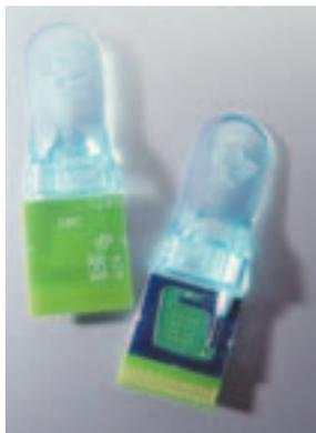
Fig. 6. Biochip de ADN eSensor™ comercializado por Motorola. Fuente: Motorola eSensor™ DNA Detection System ([http://www.motorola.com/lifesciences/esensor/tech\\_biochips.html](http://www.motorola.com/lifesciences/esensor/tech_biochips.html)).
